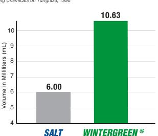
Ice melting comparisons are measured in milliliters using testing methods established by SHRP H-205.1 at 15°F for 20 minutes.
